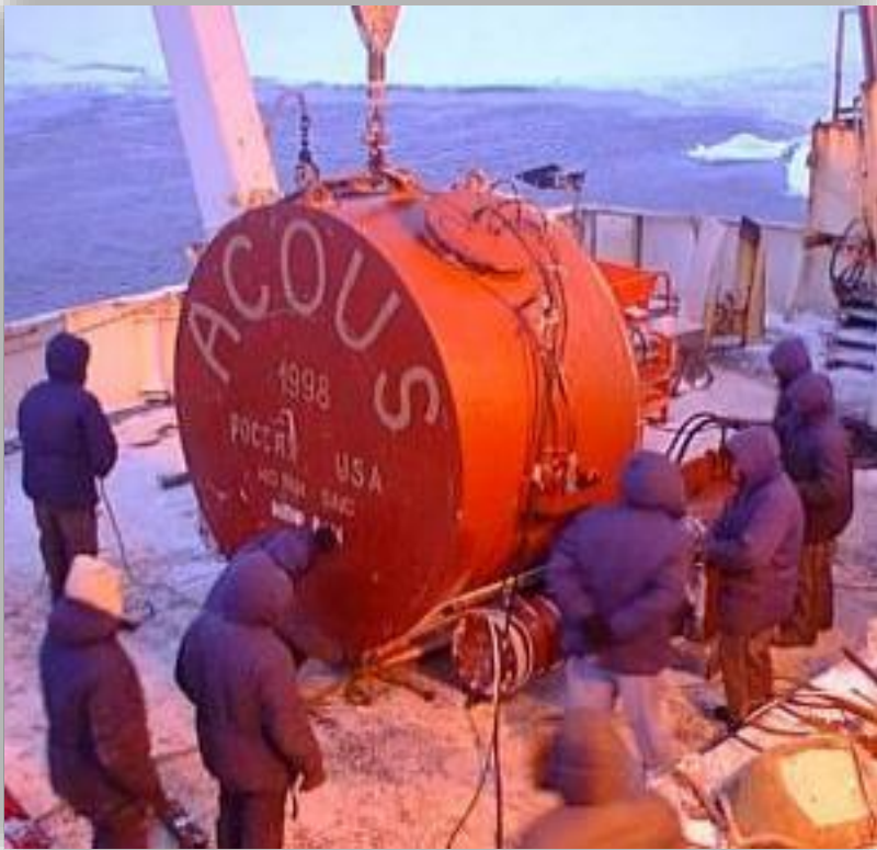
Mikhalevsky's 20 Hz, 195 dB source demonstrated transmission ranges exceeding 2,000km in 1994 and 1998.
