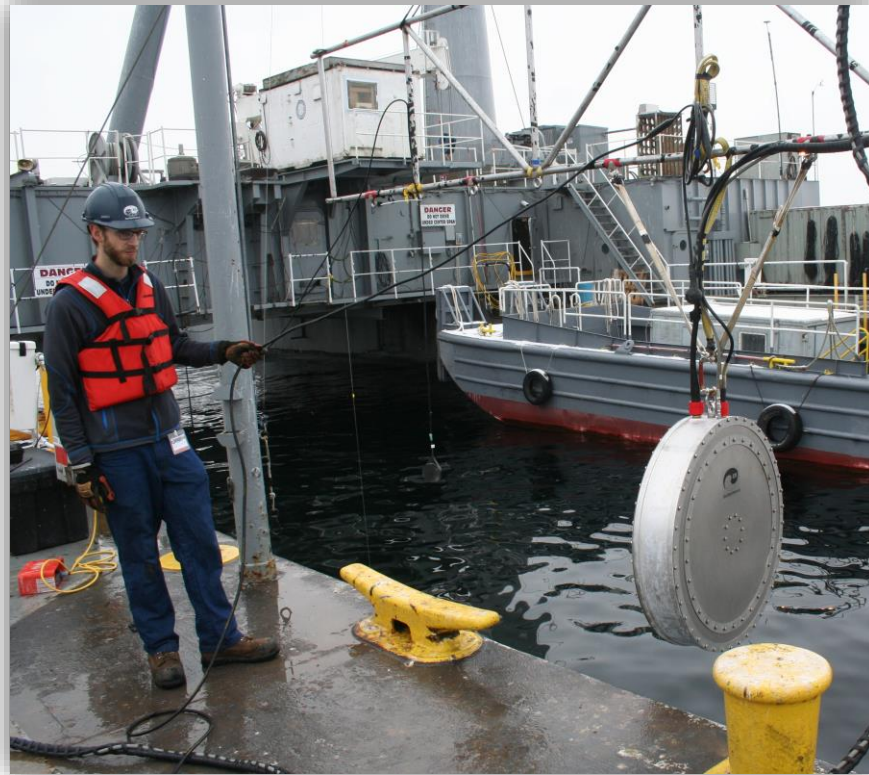
GTI 35 Hz, 195 dB source at Seneca Lake, 2017 (1 st generation) Now 200 dB at 20 Hz.
